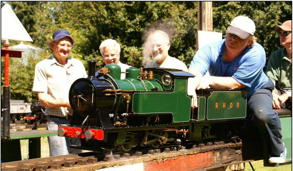
Romney Hythe and Dymchurch Railway by Kraus in 1926. The original engine left Kent in 1933 and ended up in a Belfast scrap yard, brought back to the RH&DR and was restored in the mid-1970's. During the restoration two 5" models of this engine were built alongside and one of them visited us with members of the Maidstone Club in 2007. The engine has unusual outside Stephenson link motion.
