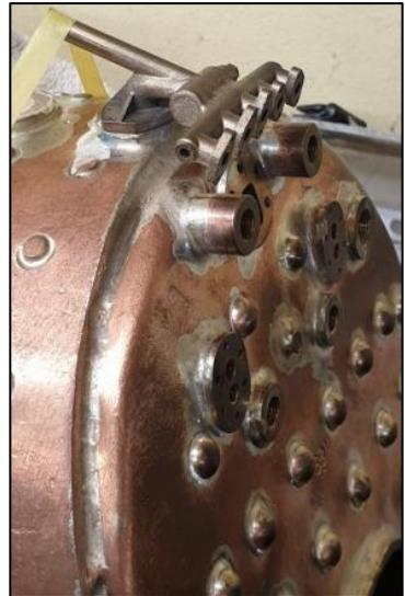
And sitting on boiler, Paul has fitted 4 blind bushes into the backhead for me to secure the cladding when done, this will be very much to scale.
