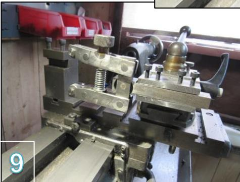
Photo 9 shows the Knurling tool in place.
