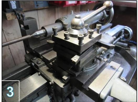
Upon receiving the drawing and material I realised that there is a modification to be made to the lathe topslide itself. So, it took time and another stab from the 4-tool turret before I started work on the tool post. It is actually only a couple of holes in the topslide for the indexing pin. Not really much of a modification at all.
